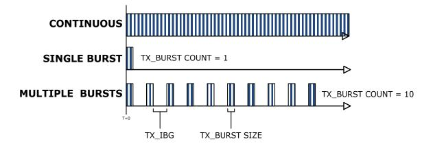
The stream transmit rate can be set using **apgSetStream CONFIG**. The stream rate can be set as in percent, packets per second or clock cycles.
