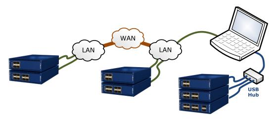
All accessible units can be managed through the same Control Interface or TCL scripting interface. The APG TCL API and the APG Control Interface share the same API to the Axtrinet Packet Generator:
