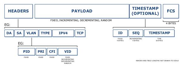
The payload can be fixed, or incrementing, decrementing or random over a range using apgSetStream PAYLOAD.
