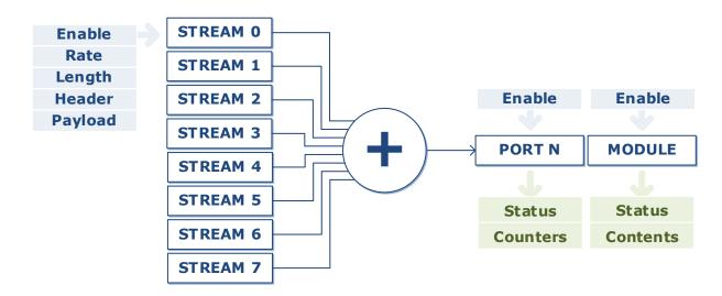
The streams are processed in a round-robin sequence, transmitting a packet if it queued and ready to send.
