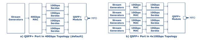
Switching between 40Gbps and 4x10Gbps topologies is performed with the **apgSetPort TOPOLOGY** command.
