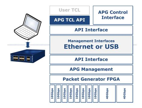
The Axtrinet APG API provides a TCL scripting interface for automated test generation.
