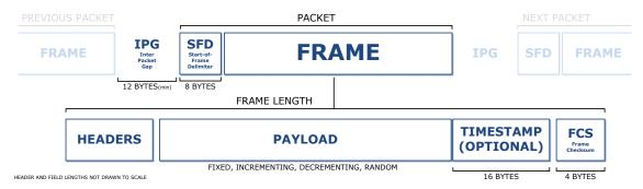
A transmit stream generates a controlled number of Ethernet frames at a controlled length and rate; with a fixed header configuration, fixed or varying header contents, and a fixed or varying payload.
