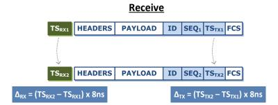
The SEQUENCE numbers are checked for out-of-order packets, gaps and repeated values.
