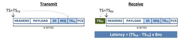
Transmit-to-transmit timing (transmit stability) and receive-to-receive timing (receiver stability) are also performed:
