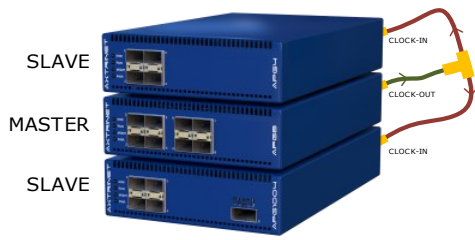
a) Multiple APG units synchronised locally
