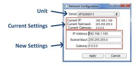
Set the IP Address, Mask and Gateway Address, then click APPLY
